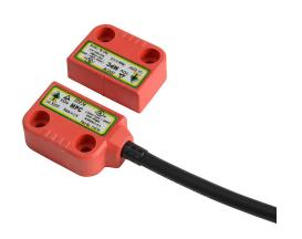
IDEM safety switch set, non-contact coded magnetic, left exit mount, (2) N.C. safety output(s), (1) N.O. monitoring output(s), plastic housing, 36 x 26mm, 8-pin M12 quick-disconnect, 9.8in/250mm cable length.
