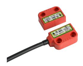
IDEM safety switch set, non-contact coded magnetic, right exit mount, (2) N.C. safety output(s), (1) N.O. monitoring output(s), plastic housing, 36 x 26mm, 8-pin M12 quick-disconnect, 9.8in/250mm cable length.
