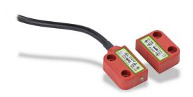
IDEM safety switch set, non-contact coded magnetic, right exit mount, (2) N.C. safety output(s), (1) N.O. monitoring output(s), plastic housing, 36 x 26mm, pigtail, 32.8ft/10m cable length.
