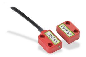
IDEM safety switch set, non-contact coded magnetic, right exit mount, (2) N.C. safety output(s), (1) N.O. monitoring output(s), plastic housing, 36 x 26mm, pigtail, 16.4ft/5m cable length.
