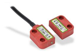
IDEM safety switch set, non-contact coded magnetic, right exit mount, (2) N.C. safety output(s), (1) N.O. monitoring output(s), plastic housing, 36 x 26mm, pigtail, 6.5ft/2m cable length.
