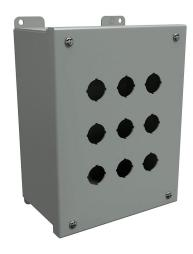
Hammond pushbutton enclosure, 9 holes, 22mm, NEMA 12/13, 9 x 7 x 4.5in (HxWxD), wall mount, carbon steel, ANSI 61 gray, powder coat finish, screw cover.
