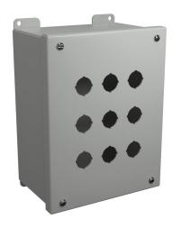
Hammond pushbutton enclosure, 9 holes, 22mm, NEMA 12/13, 9 x 7 x 4in (HxWxD), 9 x 7 x 4inmm (HxWxD), wall mount, carbon steel, RAL 7035 light gray, powder coat finish, screw cover.
