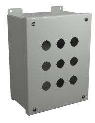
Hammond pushbutton enclosure, 9 holes, 22mm, NEMA 12/13, 9 x 7 x 4in (HxWxD), 9 x 7 x 4inmm (HxWxD), wall mount, carbon steel, RAL 7035 light gray, powder coat finish, screw cover.
