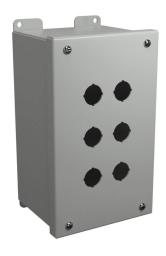
Hammond pushbutton enclosure, 6 holes, 22mm, NEMA 12/13, 9 x 5 x 4in (HxWxD), 9 x 5 x 4inmm (HxWxD), wall mount, carbon steel, RAL 7035 light gray, powder coat finish, screw cover.
