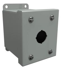
Hammond pushbutton enclosure, 1 hole, 22mm, NEMA 12/13, 4 x 3 x 4in (HxWxD), wall mount, carbon steel, ANSI 61 gray, powder coat finish, screw cover.
