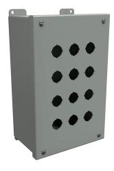
Hammond pushbutton enclosure, 12 holes, 22mm, NEMA 12/13, 11 x 7 x 4.5in (HxWxD), wall mount, carbon steel, ANSI 61 gray, powder coat finish, screw cover.
