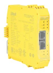
ReeR MOSAIC safety expansion module, 24 VDC, (2) TTL incremental (line driver) encoder input, (2) proximity sensor input(s), pluggable screw terminals. For use with MOSAIC-M1 and MOSAIC-M1S safety controllers.
