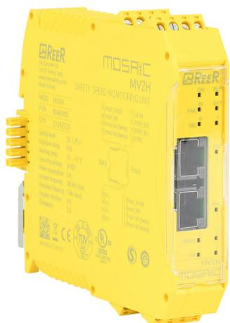
ReeR MOSAIC safety expansion module, 24 VDC, (2) HTL incremental (push-pull) encoder input, (2) proximity sensor input(s), pluggable screw terminals. For use with MOSAIC-M1 and MOSAIC-M1S safety controllers.
