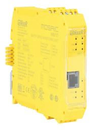
ReeR MOSAIC safety expansion module, 24 VDC, (1) TTL incremental (line driver) encoder input, (2) proximity sensor input(s), pluggable screw terminals. For use with MOSAIC-M1 and MOSAIC-M1S safety controllers.
