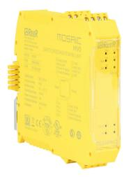
ReeR MOSAIC safety expansion module, 24 VDC, (2) proximity sensor input(s), pluggable screw terminals. For use with MOSAIC-M1 and MOSAIC-M1S safety controllers.
