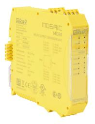
ReeR MOSAIC safety expansion module, 24 VDC, (4) EDM/ (re)start input(s), (4) N.O. safety output(s), pluggable screw terminals. For use with MOSAIC-M1 and MOSAIC-M1S safety controllers.
