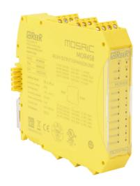
ReeR MOSAIC safety expansion module, 24 VDC, (4) EDM/ (re)start input(s), (4) N.O. safety output(s), (8) status monitoring output(s), pluggable screw terminals. For use with MOSAIC-M1 and MOSAIC-M1S safety controllers.
