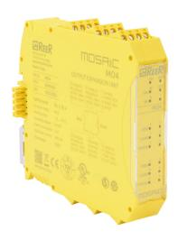
ReeR MOSAIC safety expansion module, 24 VDC, (4) EDM/ (re)start input(s), (4) pair OSSD safety output(s), (4) status monitoring output(s), pluggable screw terminals. For use with MOSAIC-M1 and MOSAIC-M1S safety controllers.
