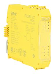
ReeR MOSAIC safety expansion module, 24 VDC, (4) Single or (2) pair OSSD safety output(s), (4) EDM/(re)start or output status configurable I/O, pluggable screw terminals. For use with MOSAIC-M1S safety controller.
