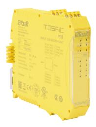
ReeR MOSAIC safety expansion module, 24 VDC, (8) digital safety input(s), pluggable screw terminals. For use with MOSAIC-M1 and MOSAIC-M1S safety controllers.
