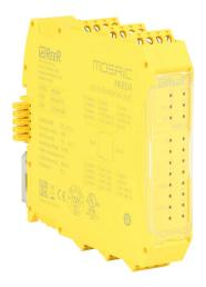
ReeR MOSAIC safety expansion module, 24 VDC, (8) digital safety input(s), (4) Single or (2) pair OSSD safety output(s), (4) EDM/ (re)start or output status configurable I/O, pluggable screw terminals. For use with MOSAIC-M1S safety controller.
