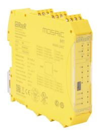
ReeR MOSAIC master safety controller, 24 VDC, (8) digital safety input(s), (2) EDM/(re)start input(s), (2) pair OSSD safety output(s), (2) status monitoring output(s), pluggable screw terminals.
