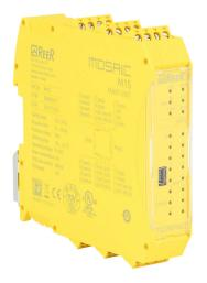
ReeR MOSAIC enhanced master safety controller, 24 VDC, (8) digital safety input(s), (4) Single or (2) pair OSSD safety output(s), (4) EDM/(re)start or output status configurable I/O, pluggable screw terminals.
