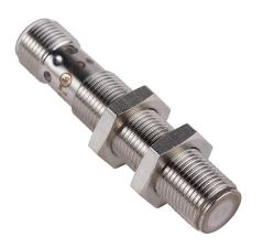
AutomationDirect magnetic proximity sensor, tubular, 12mm diameter x 60mm body, 316L stainless steel housing, PNP, N.C. output, 60mm sensing distance, flush, 5 kHz switching frequency, IP65 IP67, 4-pin M12 quick-disconnect.
