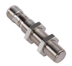
AutomationDirect magnetic proximity sensor, tubular, 12mm diameter x 60mm body, 316L stainless steel housing, PNP, N.O. output, 60mm sensing distance, flush, 5 kHz switching frequency, IP65 IP67, 4-pin M12 quick-disconnect.
