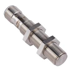
AutomationDirect magnetic proximity sensor, tubular, 12mm diameter x 60mm body, 316L stainless steel housing, NPN, N.O. output, 60mm sensing distance, flush, 5 kHz switching frequency, IP65 IP67, 4-pin M12 quick-disconnect.
