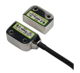
IDEM safety switch set, non-contact magnetic, left exit mount, (2) N.C. safety output(s), (1) N.O. monitoring output(s), 316 stainless steel housing, 36 x 26mm, 8-pin M12 quick-disconnect, 9.8in/250mm cable length.
