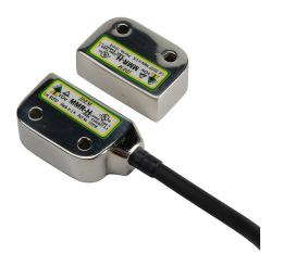
IDEM safety switch set, non-contact magnetic, left exit mount, (2) N.C. safety output(s), (1) N.O. monitoring output(s), 316 stainless steel housing, 36 x 26mm, 8-pin M12 quick-disconnect, 9.8in/250mm cable length.
