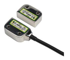
IDEM safety switch set, non-contact magnetic, left exit mount, (2) N.C. safety output(s), (1) N.O. monitoring output(s), 316 stainless steel housing, 36 x 26mm, pigtail, 32.8ft/10m cable length.
