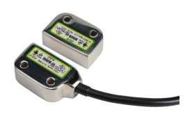
IDEM safety switch set, non-contact magnetic, left exit mount, (2) N.C. safety output(s), (1) N.O. monitoring output(s), 316 stainless steel housing,  $36 \times 26$ mm, pigtail, 16.4ft/5m cable length.
