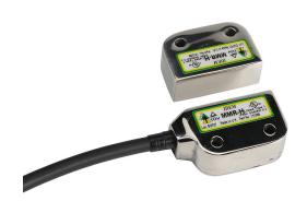
IDEM safety switch set, non-contact magnetic, right exit mount, (2) N.C. safety output(s), (1) N.O. monitoring output(s), 316 stainless steel housing, 36 x 26mm, 8-pin M12 quick-disconnect, 9.8in/250mm cable length.
