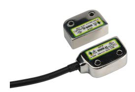
IDEM safety switch set, non-contact magnetic, right exit mount, (2) N.C. safety output(s), (1) N.O. monitoring output(s), 316 stainless steel housing, 36 x 26mm, pigtail, 16.4ft/5m cable length.
