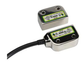
IDEM safety switch set, non-contact magnetic, right exit mount, (2) N.C. safety output(s), (1) N.O. monitoring output(s), 316 stainless steel housing, 36 x 26mm, pigtail, 6.5ft/2m cable length.
