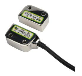
IDEM safety switch set, non-contact coded magnetic, left exit mount, (2) N.C. safety output(s), (1) N.O. monitoring output(s), 316 stainless steel housing, 36 x 26mm, pigtail, 16.4ft/5m cable length.
