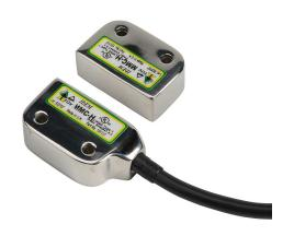
IDEM safety switch set, non-contact coded magnetic, left exit mount, (2) N.C. safety output(s), (1) N.O. monitoring output(s), 316 stainless steel housing, 36 x 26mm, pigtail, 6.5ft/2m cable length.
