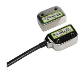
IDEM safety switch set, non-contact coded magnetic, right exit mount, (2) N.C. safety output(s), (1) N.O. monitoring output(s), 316 stainless steel housing, 36 x 26mm, pigtail, 32.8ft/10m cable length.
