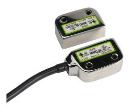
IDEM safety switch set, non-contact coded magnetic, right exit mount, (2) N.C. safety output(s), (1) N.O. monitoring output(s), 316 stainless steel housing, 36 x 26mm, pigtail, 16.4ft/5m cable length.
