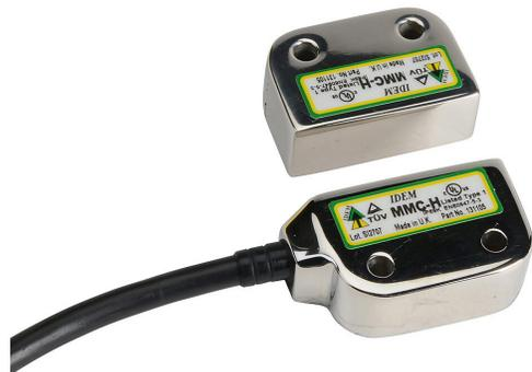
IDEM safety switch set, non-contact coded magnetic, right exit mount, (2) N.C. safety output(s), (1) N.O. monitoring output(s), 316 stainless steel housing, 36 x 26mm, pigtail, 6.5ft/2m cable length.
