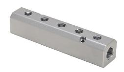
NITRA pneumatic valve manifold, aluminum, rectangular, 500 psi maximum operating pressure, (5) stations, (2) 1/2in female NPT inlet(s), (5) 1/4in female NPT outlet(s), standard hole spacing.
