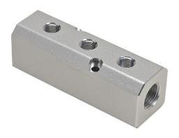
NITRA pneumatic valve manifold, aluminum, silver, rectangular, 500 psi maximum operating pressure, (3) stations, (2) 1/2in female NPT inlet(s), (3) 1/4in female NPT outlet(s), standard hole spacing.
