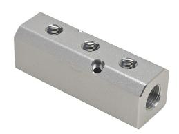
NITRA pneumatic valve manifold, aluminum, rectangular, 500 psi maximum operating pressure, (3) stations, (2) 1/2in female NPT inlet(s), (3) 1/4in female NPT outlet(s), standard hole spacing.
