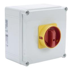
Merz rotary enclosed disconnect switch, load break capable, 3-pole, 600 VAC, 125A, 5kA SCCR, wall mount, UL 508 rated,  $7.8 \times 7.8 \times 6.4$ in housing.
