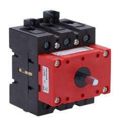
Merz manual motor controller, open, 125A, 600 VAC, 3-pole, 50hp, 35mm DIN rail or panel mount, UL 508 rated.
