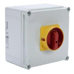
Merz rotary enclosed disconnect switch, load break capable, 3-pole, 600 VAC, 63A, 5kA SCCR, wall mount, UL 508 rated,  $7.8 \times 7.8 \times 6.4$ in housing.
