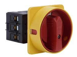
Merz rotary disconnect switch, load break capable, 3-pole, 600 VAC, 63A, 5kA SCCR, door mount, UL 508 rated, front operated. Hardware for 4-hole door mounting & lockable red/yellow handle for use with NEMA 4/4X enclosures included.
