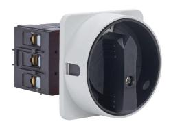
Merz rotary disconnect switch, load break capable, 3-pole, 600 VAC, 63A, 5kA SCCR, door mount, UL 508 rated, front operated. Hardware for 4-hole door mounting & lockable black/gray handle for use with NEMA 4/4X enclosures included.
