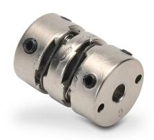
AutomationDirect encoder coupling, 4mm to 1/4in bore, aluminum alloy body, setscrew. For use with Koyo TRD-MX series encoders and NEMA size 23 stepper motors.
