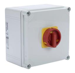
Merz rotary enclosed disconnect switch, load break capable, 3-pole, 600 VAC, 40A, 5kA SCCR, wall mount, UL 508 rated,  $7.8 \times 6.4$ in housing, switched neutral.
