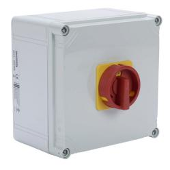
Merz rotary enclosed disconnect switch, load break capable, 3-pole, 600 VAC, 40A, 5kA SCCR, wall mount, UL 508 rated,  $7.8 \times 7.8 \times 6.4$ in housing.
