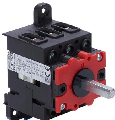
Merz manual motor controller, open, 40A, 600 VAC, 3-pole, 20hp, 35mm DIN rail or panel mount, UL 508 rated.
