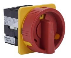
Merz rotary disconnect switch, load break capable, 3-pole, 600 VAC, 40A, 5kA SCCR, door mount, UL 508 rated, front operated. Hardware for 4-hole door mounting & lockable red/ yellow handle for use with NEMA 4/4X enclosures included.
