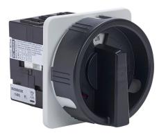
Merz rotary disconnect switch, load break capable, 3-pole, 600 VAC, 40A, 5kA SCCR, door mount, UL 508 rated, front operated. Hardware for 4-hole door mounting & lockable black/ gray handle for use with NEMA 4/4X enclosures included.
