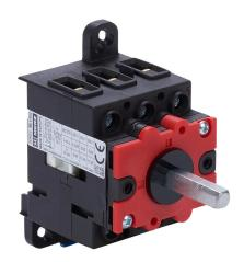
Merz manual motor controller, open, 32A, 600 VAC, 3-pole, 20hp, 35mm DIN rail or panel mount, UL 508 rated.
